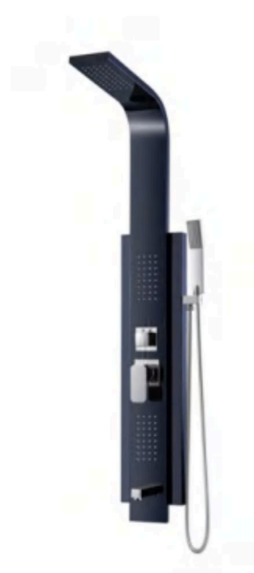
Y045B 1320*200*430mm 1.#304 stainless steel body in brush nickle finish 2.top shower 3.back massage nozzle 4.hand shower 5.Spout
